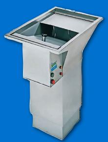
**1604** (F54/320) Capacity - 1850 covers per sitting. 900Kg waste / hour 3 Phase 4.kW (5.5HP)
