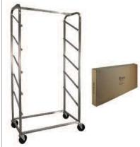
Shelves: 5 forward tilt, Shelf Spacing: 270 Capacity: 5 wire baskets Overall Dimensions: 975x1785x455 Finish: Stainless Steel
