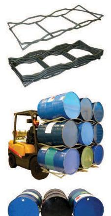
Overall Dimensions: Length: 1760 Width: 730 Height: 220 Weight: 15kg Stacks up to 5 drums high Material: 25mm outside diameter 1.6mm ERW tube & 25x6mm flat bar Surface Finish: Hot dipped galvanised
