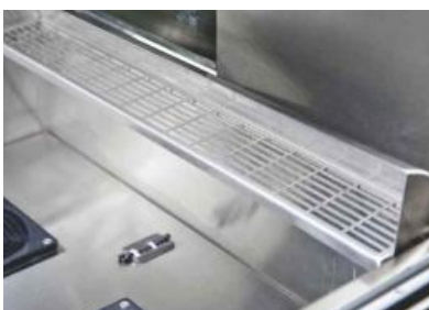
Blown air units circulate above and below the pans
